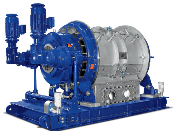
Fig. 3. Pressure filtration can also be used in chemical recycling of PET, e.g. with the rotary pressure filter RPF.
